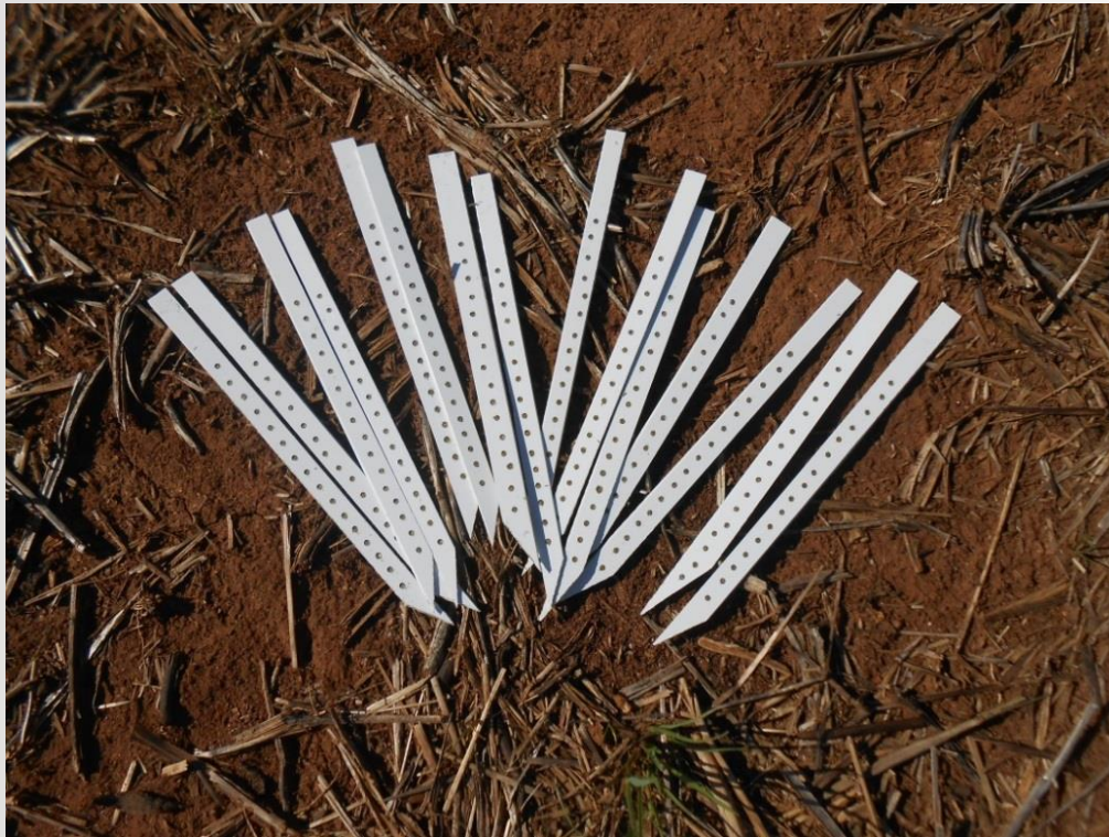
Bait lamina to determine the microbial activity in the soil (Dra. Gerusa Steffen et al.).
