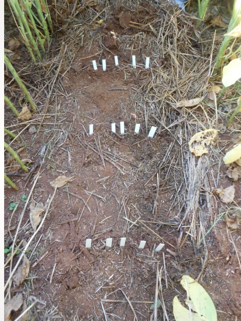
Bait lamina to determine the microbial activity in the soil (Dra. Gerusa Steffen et al.).
